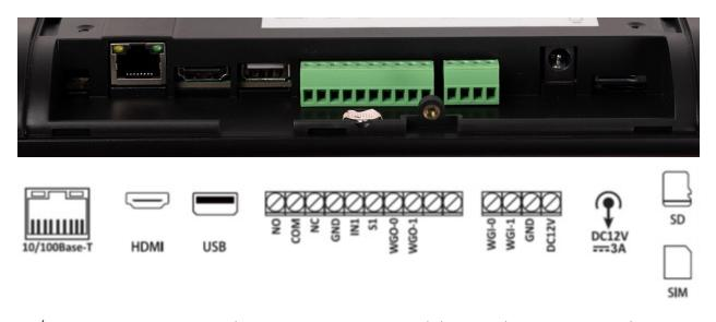
10/100Base-T: RJ-45 Ethernet connector with PoE (IEEE802.3BT) HDMI: Connect the device to an external monitor. Strip 1: Used to operate a connected electric lock. Strip 2: Used for connection to an external reader. DC12V: Connection to 12V DC, 3A power supply. SD: SD card slot for additional storage. Press ''ESC' on the smart terminal to check the capacity of the SD card. SIM: SIM card slot for units that feature 4G operation.
